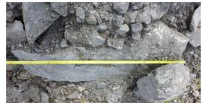
Picture 8: Subsurface material – up to 1m diameter
