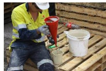
Picture 2: Viscosity Testing
