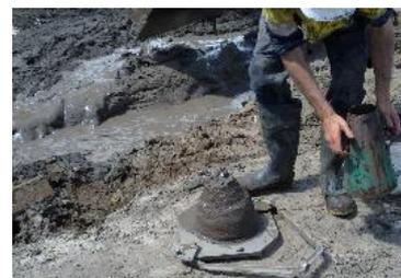
Picture 1: Slump Testing
