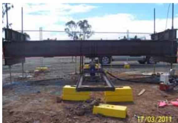
Figure 10. Site photo of the static load testing setup.
