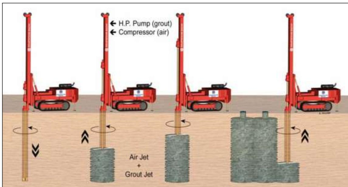
*Figure 6: Jet grouting procedure*
