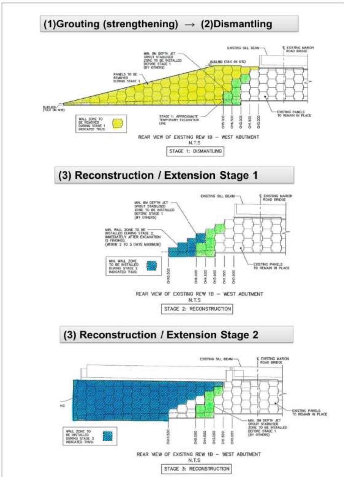
**Figure 1: Typical RE bridge abutment duplication staging**
