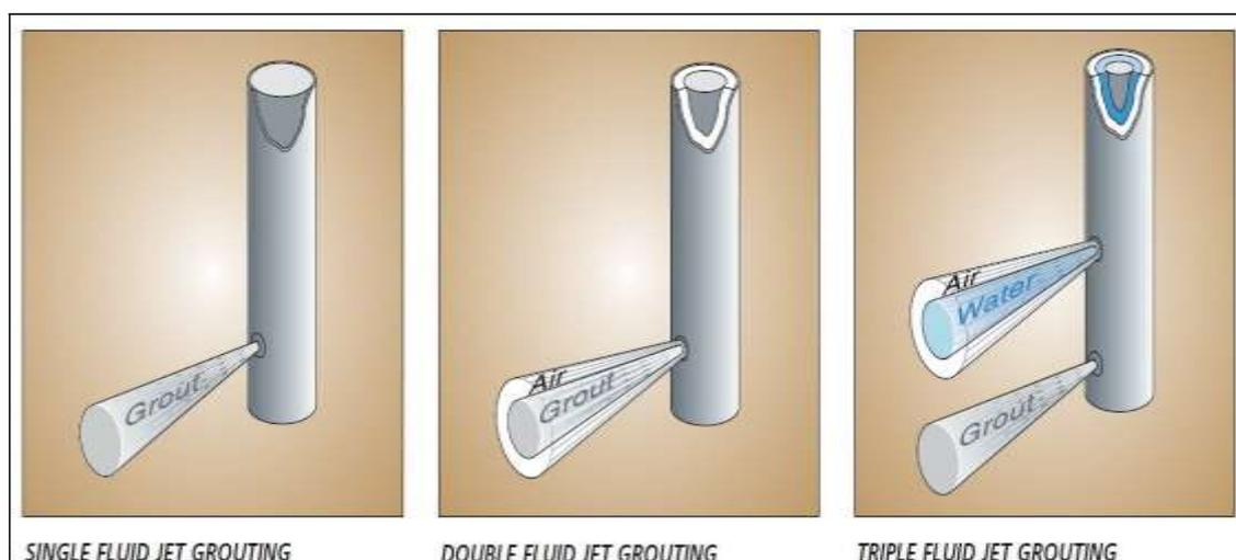
**Figure 7: The three most common Jet Grouting Systems**
