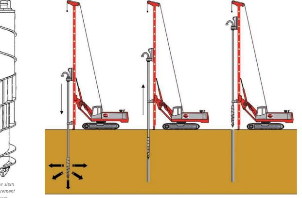
Hollow stem displacement auger
