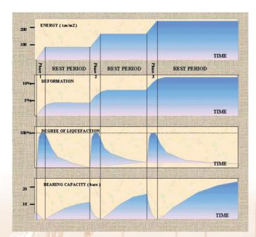
During Dynamic Compaction, an immediate effect and a differed phenomenon can usually be distinguished:
